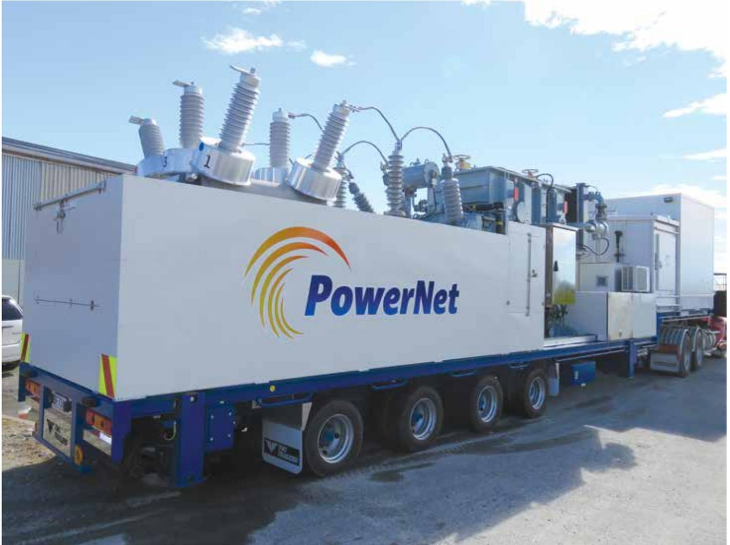
ABB's technology is part of PowerNet's latest mobile substation solution which is geared to support continuity of supply.
