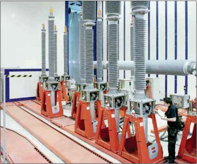
18 Routine Tests Live Tank Circuit Breaker
