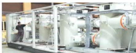
Integrated GIS, 145 - 420 kV
