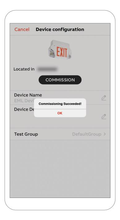
After pressing OK, the screen will open the floor map you set at the "Configuring the buildings of the organization" step. An image of the device will appear on the map. By clicking on the map, the image of the device can be dragged and dropped to set the location of the device on the floor plan.
