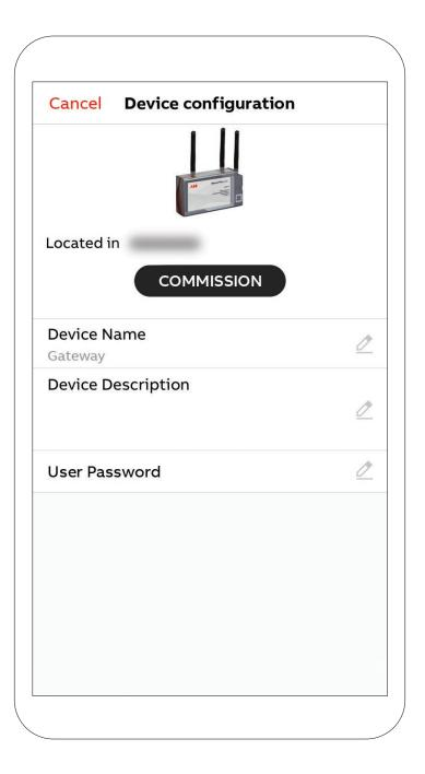
After filling the page and pressing the Commission button, the iOS device will send the proper configuration to the Gateway. During this step, it is important to stay within the vicinity of the Gateway. Once the following pop-up appears, the configuration is completed.
