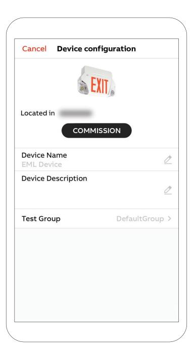
When you have completed filling in the information, press the Commission button. The iOS device will send the proper configuration to the unit. During this step, it is important to stay within the vicinity of the unit. Once the following pop-up appears, the configuration is completed.
