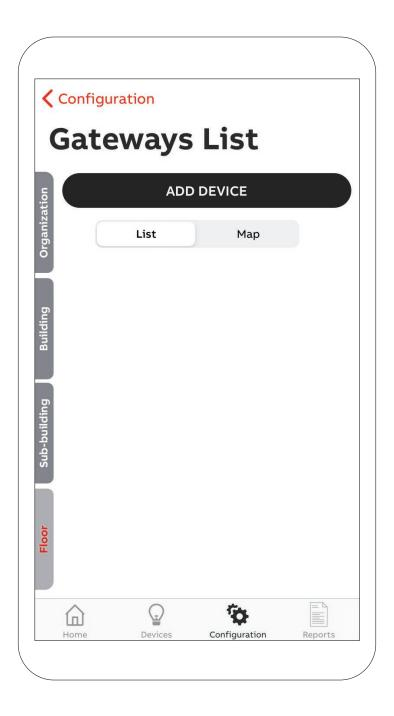
Once you press the Add Gateway button, your smart phone or tablet camera turns on and asks to scan the QR code located on the Gateway. Make sure the Gateway is plugged in.
