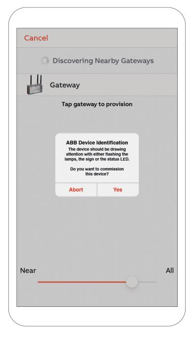
If a floor plan was loaded, the Gateway can be placed on a floor plan, otherwise the screen will transition directly to the Device Configuration page. A name and description can be given to that Gateway. It is also mandatory to enter the login user password, to enable cloud access.
