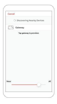
After selecting a Gateway from the list, the LED's on the selected Gateway will start flashing and a pop-up will appear on the app requiring validation.
