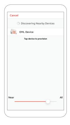
After selecting the device from the list, it should start flashing or turn on. A pop-up will appear in the app asking for confirmation.
