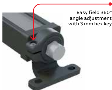
A - Adjustable mounting bracket (optional)
