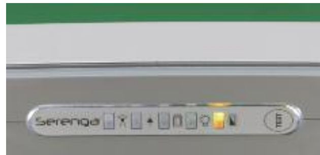
Amber LED indicates a fault.
