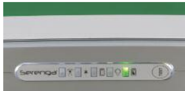
Green LED indicates normal operation.
