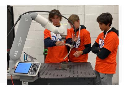
ABB's Cobot Arc Welding STEM Education Cell is designed to maximize the required training needs to master robotic welding programming, electrical service, mechanical maintenance, and offline/on-line software packages. All educational software packages are included with the robot.
