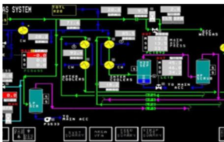
**Figure 3.** Older highly colored screens with symbolic representations of control logic make it difficult for operators to focus in on the locations and values of alarm conditions.
