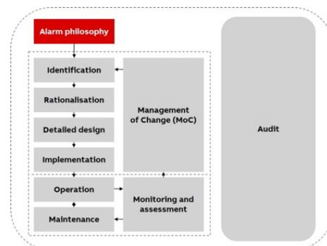
**Figure 2.** Good alarm lifecycle management starts with a sound philosophy that prioritizes alarm hierarchies and establishes a process for continuous review and improvement.
